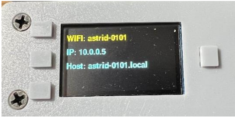
Mini-display showing Astrid broadcasting its own hotspot SSID
