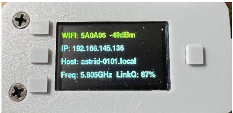
Mini-display showing Astrid connected to a home network
