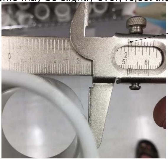
Slightly under 2" outside diameter, measured near center. The other end of the large couplings might have one small embossed number. Just sand or scrape this number down smooth.
