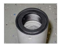
Now you can insert the carrier into your 2" drawtube far enough to allow the camera + focal reducer to come to focus, without shortening struts or moving the primary.
