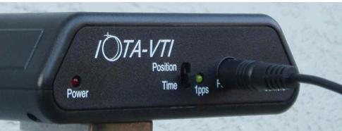
To avoid the exorbitant cost of a custom panel for this low-volume model, a hole is cut in the standard panel. Labels suffer.
