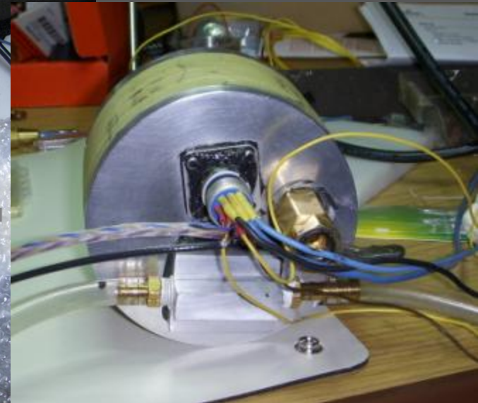
Parts - Bit-whacker controller, VCO, vacuum chamber, custom detector boards
