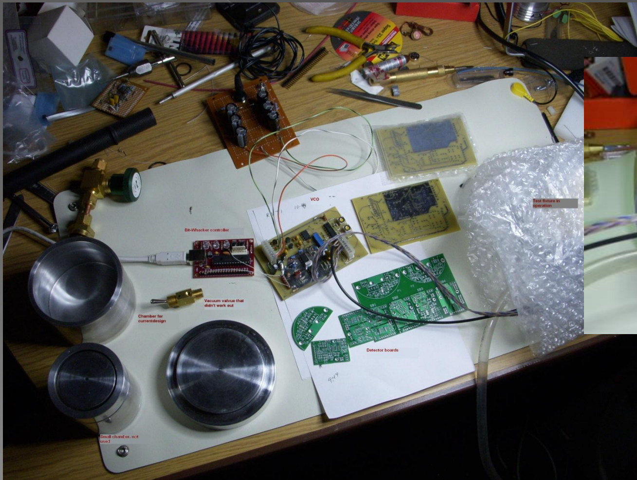
Parts - Bit-whacker controller, VCO, vacuum chamber, custom detector boards
