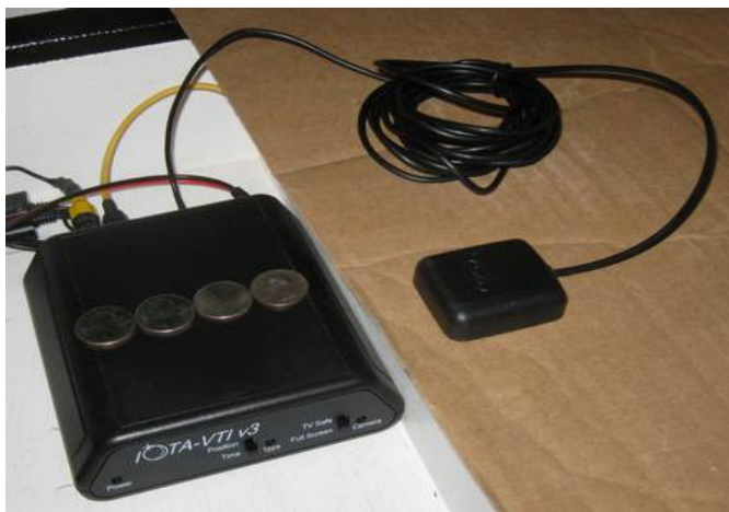
Above is an image of an IOTA VTI with its external antenna. (Note the 4 US quarters across the top as a size reference).
