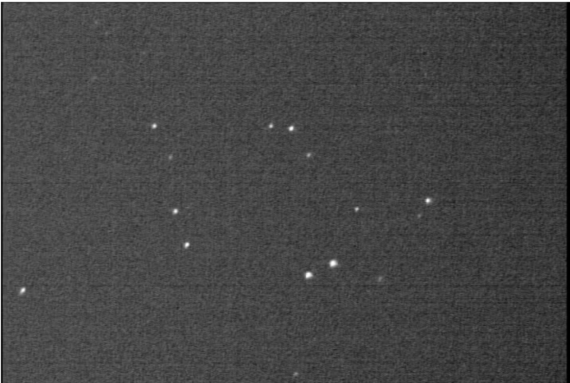
Figure 7: This used a 2016 focal reducer (reversed) and the RunCam Night Eagle camera. The “A” distance was 160mm, giving a focal reduction of 0.61, with again coma; an extension tube was needed to focus; the video file is 20170105Hyades5.avi:
