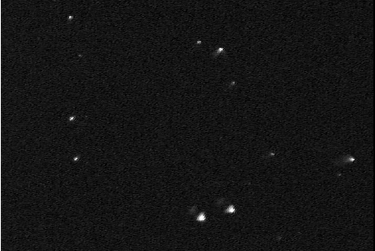
Figure 4: This used a 2016 focal reducer and the PC164C-EX2 camera. The 75 – 85 Tauri distance was 187mm, giving a focal reduction of 0.60, with noticeable coma, & ghost images for bright \theta^1 and \theta^2 Tauri; video file 20170105Hyades3.avi:
