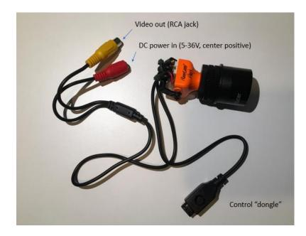
You can easily test the camera upon receipt by unscrewing the optical "stack", reinstalling the original wide angle lens, applying power, and sending the output through a standard RCA cable to the AV input on a regular television.
