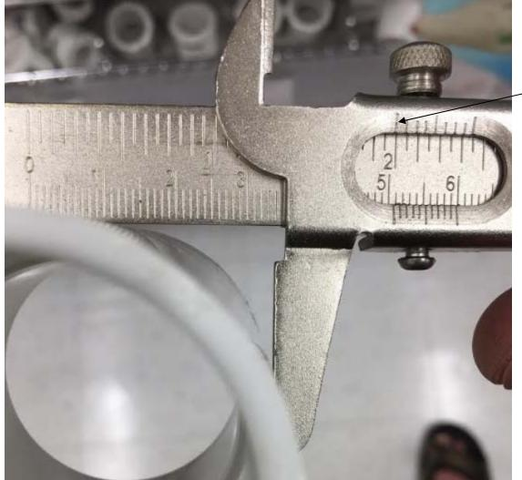
Slightly under 2" outside diameter, measured near center. The other end of the large couplings might have one small embossed number. Just sand or scrape this number down smooth.
