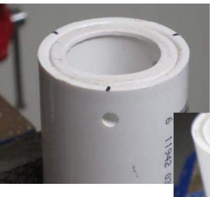
Plastic is soft, you can drive the tap in and out with a reversing drill.
