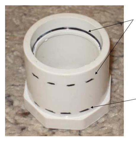
Cut through adapter even with black line to leave inner ring flush with the new cut end. This inner ring will serve as a stop for the 1 ¼" camera focal reducer.
