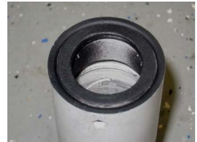
Now you can insert the carrier into your 2" drawtube far enough to allow the camera + focal reducer to come to focus, without shortening struts or moving the primary.
