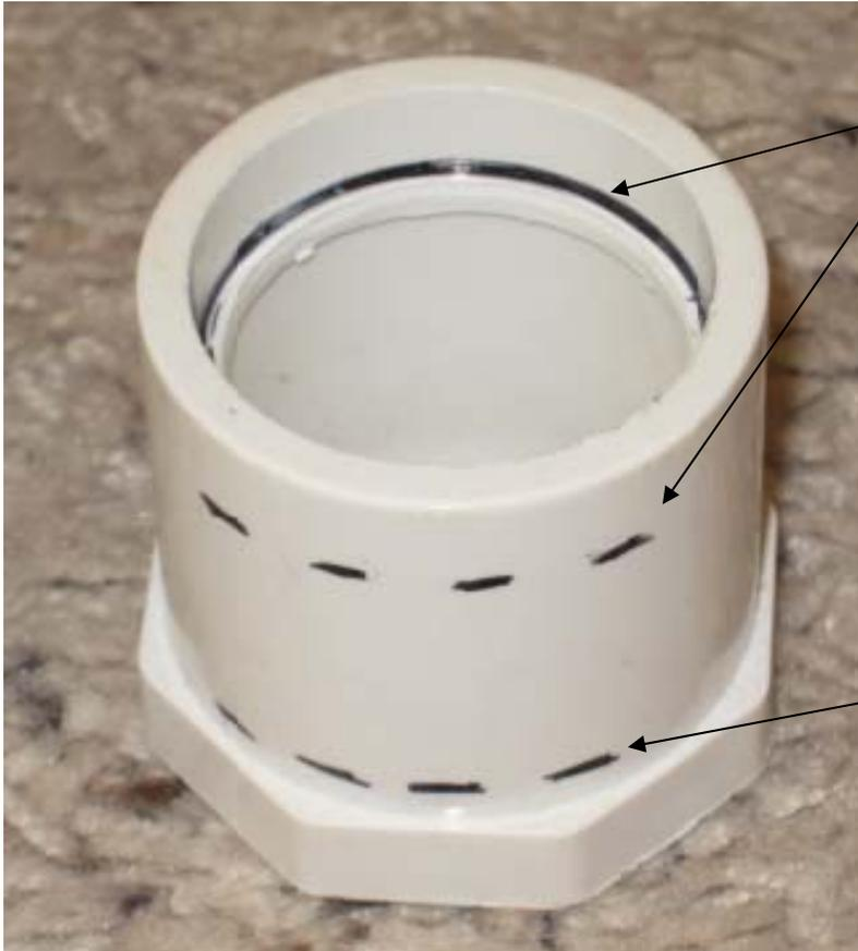
Cut through reducing bushing even with black line to leave inner ring flush with the new cut end. This inner ring will serve as a stop for the 1 ¼" camera focal reducer.
