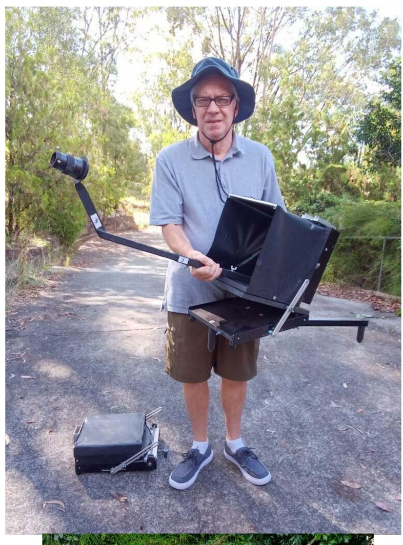
John Broughton (Reedy Creek, Australia) designs and builds portable telescopes or portable mounts for refractors expressly intended to fit into a suitcase for ease if travel. He is displaying his Wombat 250, a 10-inch reflector, that folds to a compact rectangle. His equipment and observing techniques include: Camera: WAT910-HX, RunCam, occasionally QHY174-GPS Recording equipment: mini DVRs no longer manufactured.
