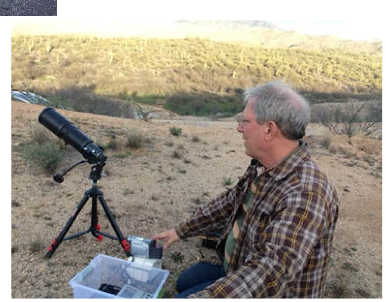
Ted Blank (Arizona USA) uses 120 or 80mm scopes on sprinkler tripods, modified with a Scotty Degenhardt design or, for fainter events, a Celestron 8 or 9.5, or a 10inch SkyWatcher Dobsonian.
